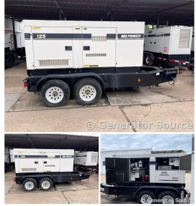
**Description:** Multiquip 100 kW Diesel Trailer Mounted Generator Model #: DCA125SSIU, Serial #: 7510466 4979 Hours, 277/480 Volt, Voltage Selector Switch Sound Attenuated Enclosure on Trailer
