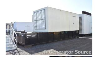
**Description:** Kohler 1500 kW Diesel Generator Model #: 1500REOZDB, Serial #: 2073065 Year 2005, 484 Hours, 480 Volt, 3 Phase, Weatherproof Enclosure
